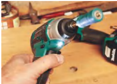
A single trigger operated LED is a handy feature on both tools
